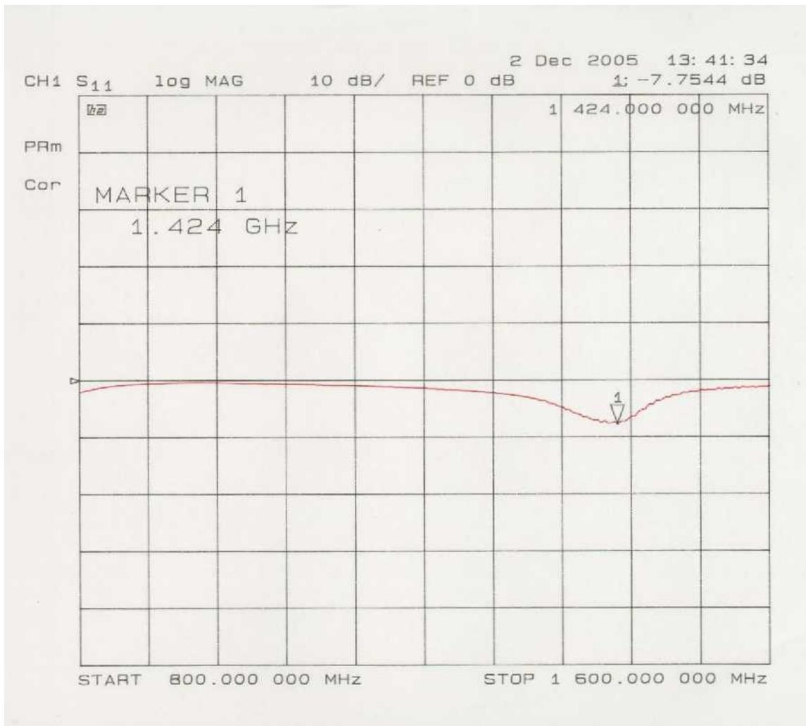
**Figure 7 Return Loss of 1.43GHz antenna**
