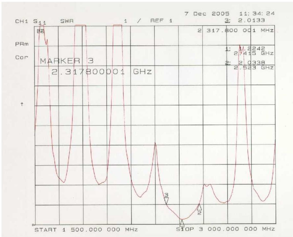
**Figure 8 VSWR of 2.4GHz Antenna**
