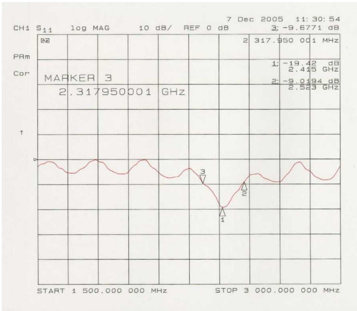
**Figure 6 Return Loss of 2.4GHz Antenna**
