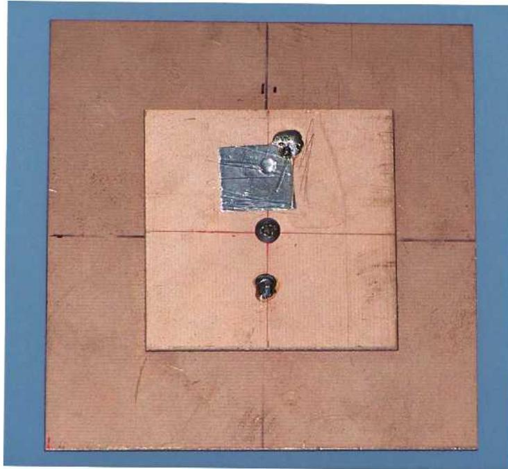
**Figure 3 Prototype 2.4GHz Antenna**
