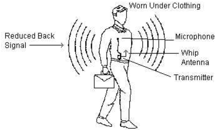
Figure 1.1 A Complete Body-Wire System
